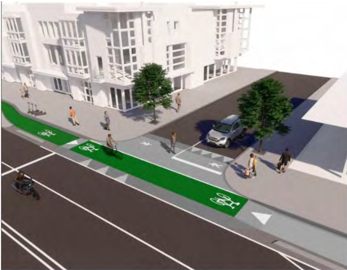
Example of side street raised table intersection.
