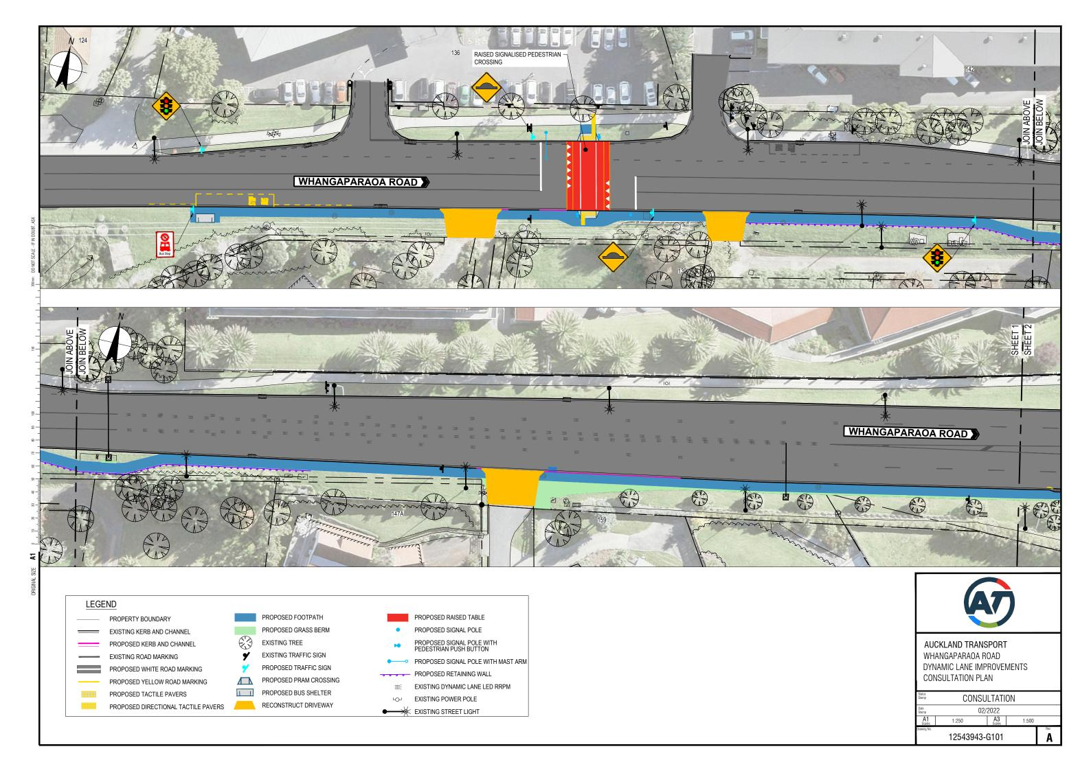
EXISTING KERB AND CHANNEL PROPOSED KERB AND CHANNEL EXISTING ROAD MARKING
