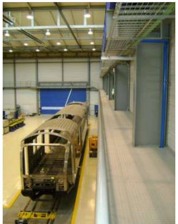
Figure 3: Bodyshell being instrumented for mechanical testing
