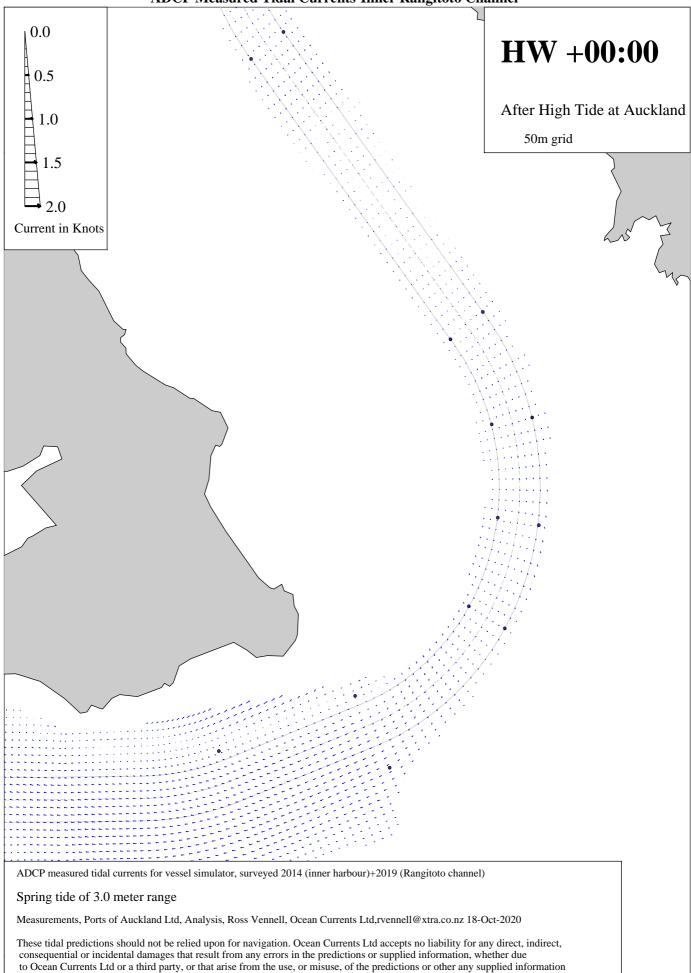
**ADCP Measured Tidal Currents-Inner Rangitoto Channel**
