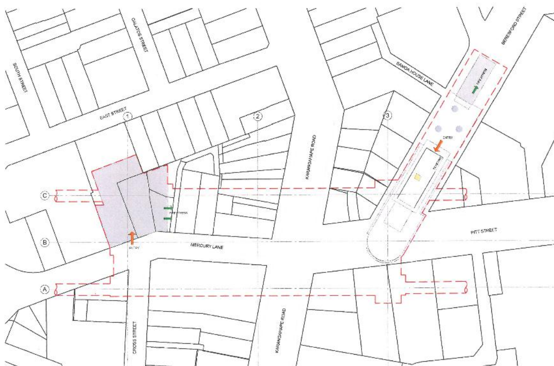
Figure 17. Karangahape Station showing top down construction areas (grey shading). From 2012 Concept Design Report
