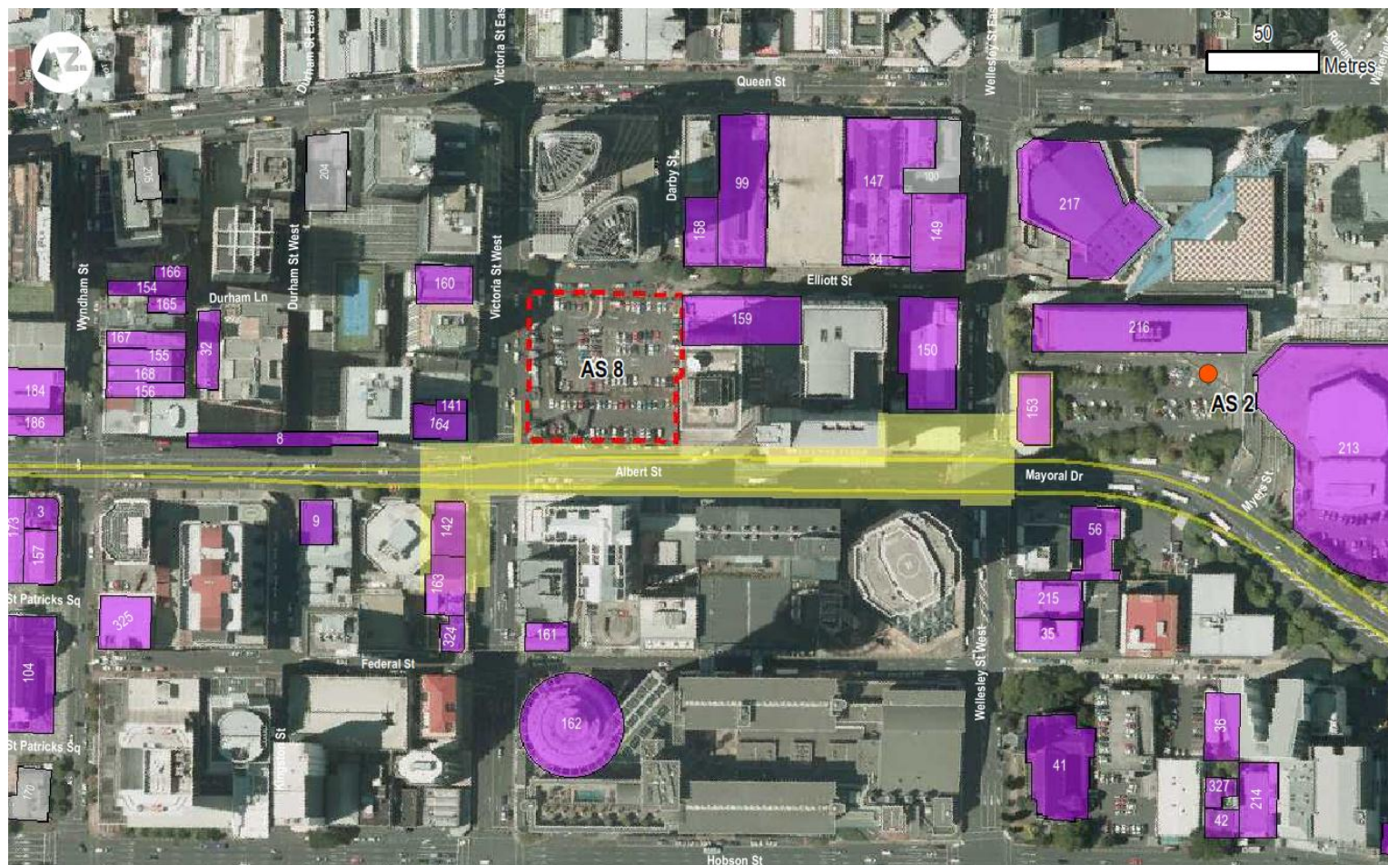
Figure 14. Plan showing the extent of the proposed Aotea Station, to be excavated, recorded heritage buildings located within close proximity (identified by BHR number, and recorded archaeological sites (AS 8)
