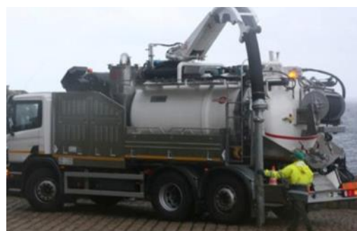
Above image: Hydro excavating truck.
