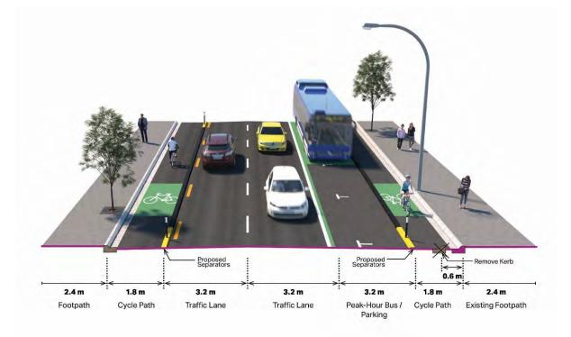
For this section we are proposing an on-road cycle lane in both directions, protected from traffic by a physical barrier.
