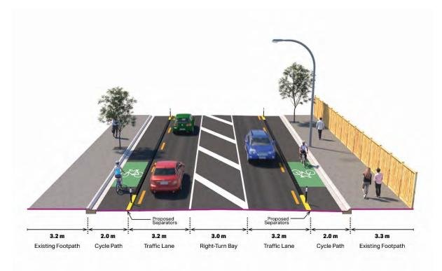
For this section, we propose an on-road cycle lane in each direction, protected from traffic by a physical barrier. Additional side street treatments will be implemented, to increase safety for all users.
