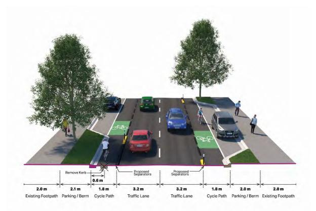
For this section, we are proposing an on-road cycle lane in each direction, protected from traffic by a physical barrier. Additional side street treatments will be implemented, to increase safety for all users.
