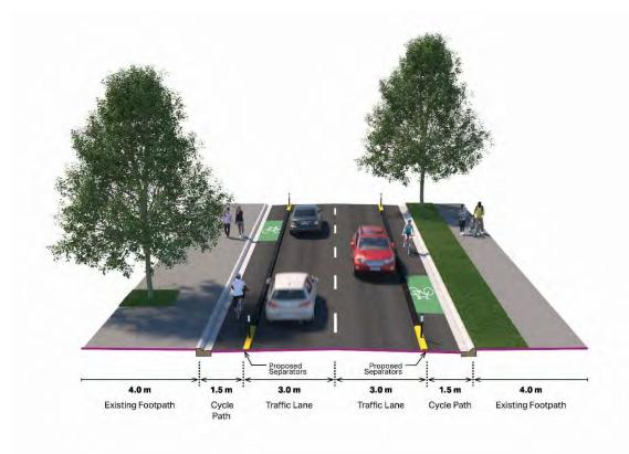
For this section, we are proposing an on-road cycle lane in each direction, separated from traffic by a physical barrier.
