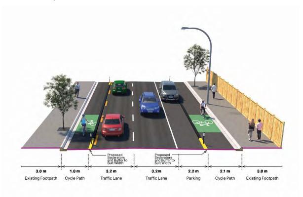
For this section we are proposing an on-road cycle lane in each direction, protected from traffic by a physical barrier. Additional side street treatments will be implemented, to increase safety for all users.
