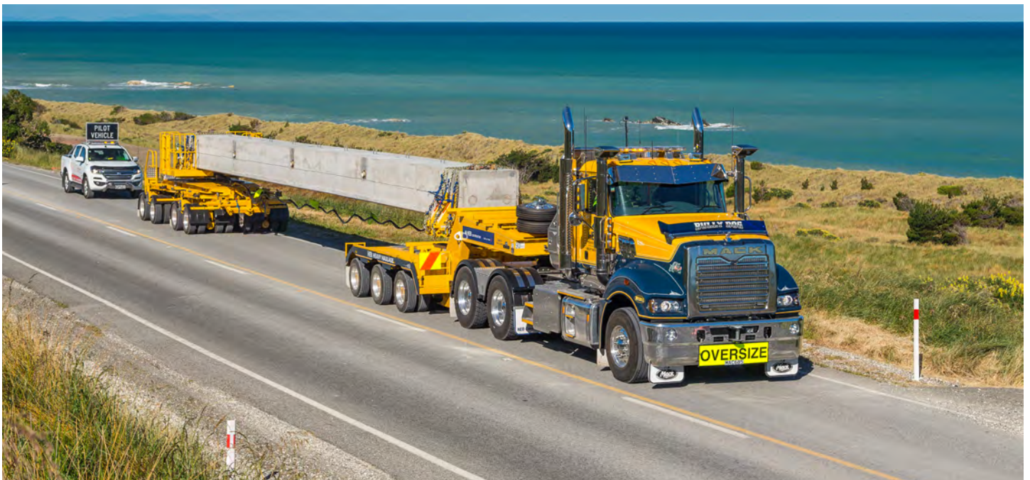
Example of the transporter to be used for the delivery of the beams
