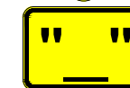
PW-17 CURVED ARROW WARNING SIGN MODIFIED WITH SIDE ROAD STICKER WITH SUPPLEMENTARY SPEED " __ " SIGN. (LEFT OR RIGHT)
