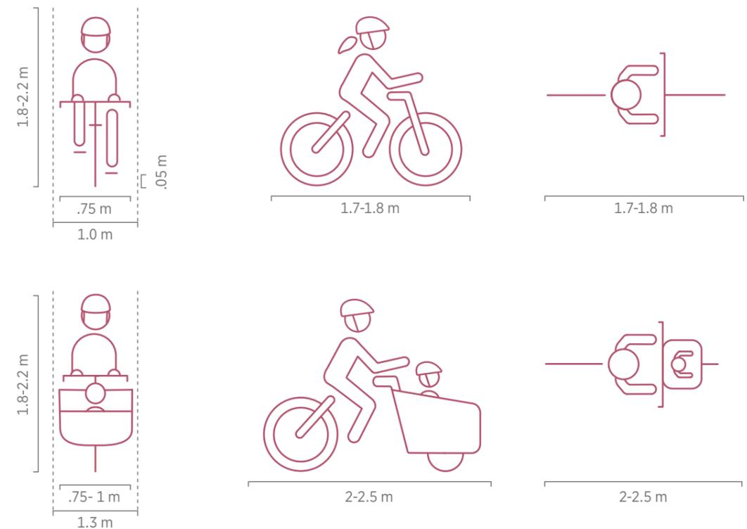
Minimum envelope for bike users is 1.0 m wide, allowing for some weaving for stability, especially uphill.
