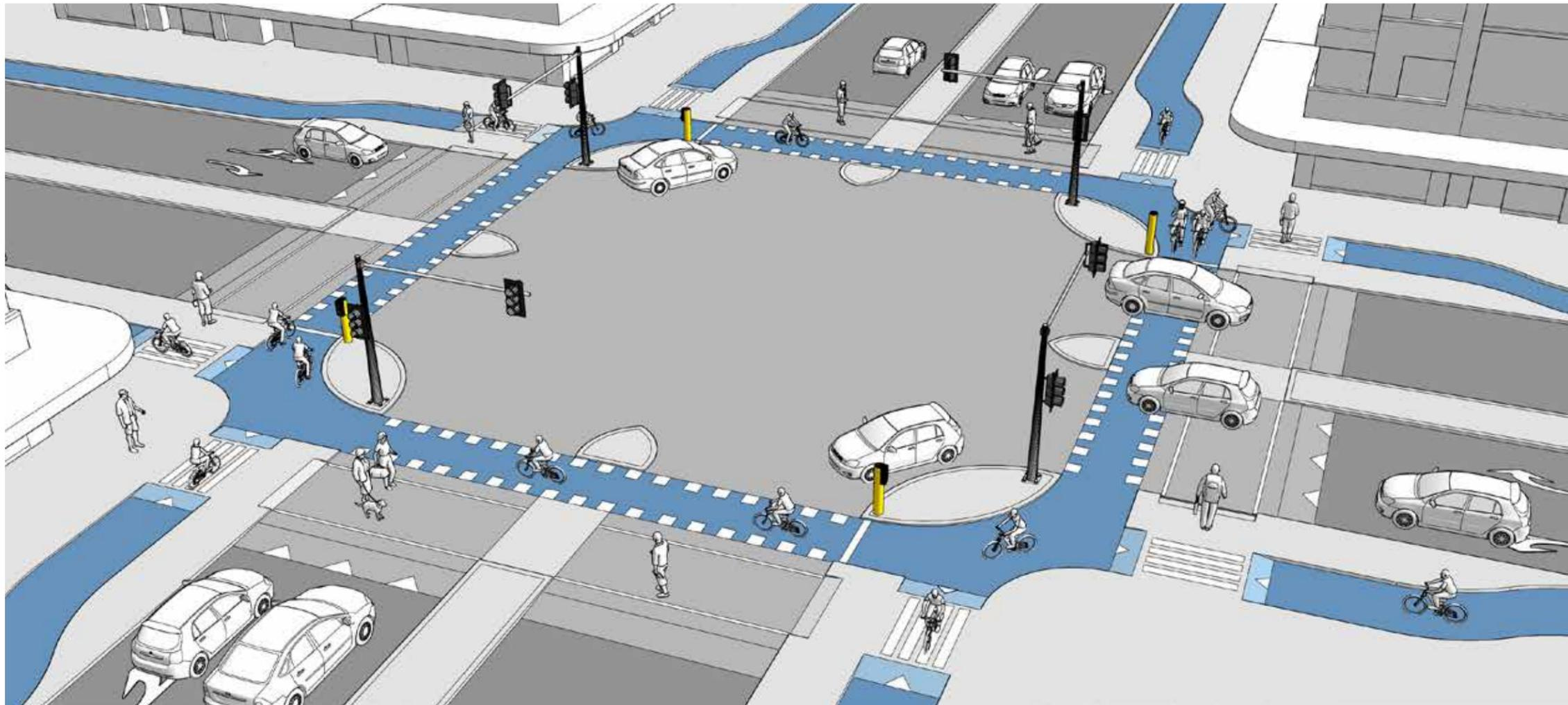
Pedestrian crossings are situated behind the cycle crossing. Pedestrians crossing the intersection first cross the cycle paths, where cyclists must give way to them. Pedestrian safety islands are provided between the cycle paths and the pedestrian crossing, which is preferably demarcated using a zebra crossing.
