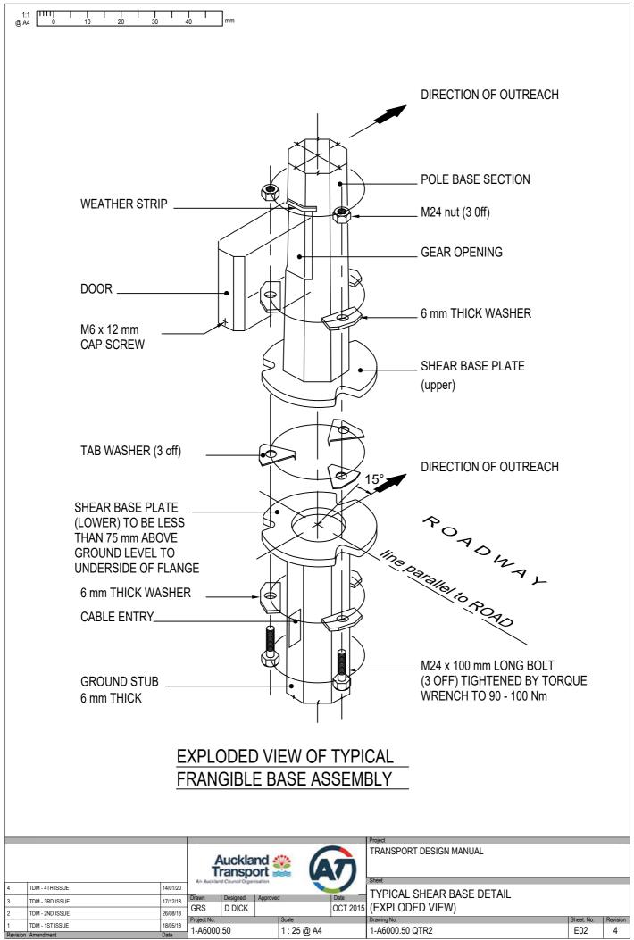
riginal Sheet Size A4 [210x297] VERSION 4\_14/01/20 TDM\_APPENDIX K4 - TYPICAL SHEAR BASE DETAIL
