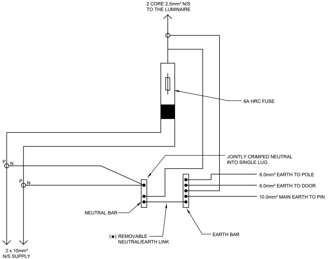
**STANDARD STREETLIGHTING POLE ELECTRICAL CONNECTIONS**
