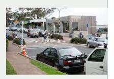
In a road with high movement function, parking has to be designed to minimise its impact on the operation of the traffic lanes. This can be done either through limiting the provision of parking, or by providing for entry and exit manoeuvres that do not impede the through traffic.
