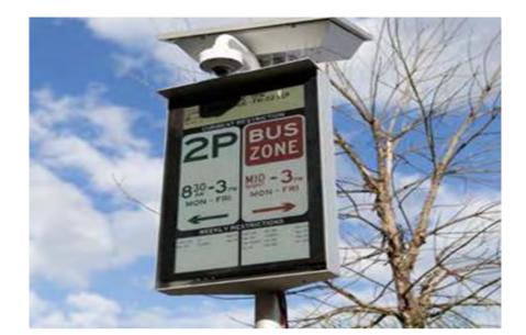
Display parking availability, restrictions, directions, pricing, and other messages in real-time. Digital signage could be supported by the use of digital line-markings to visually display changes in restrictions.
