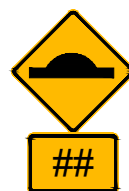
Advance warning sign W14-4 with supplementary advisory speed sign W12-3.2 to be installed on approaching speed table, speed humps or speed cushions
