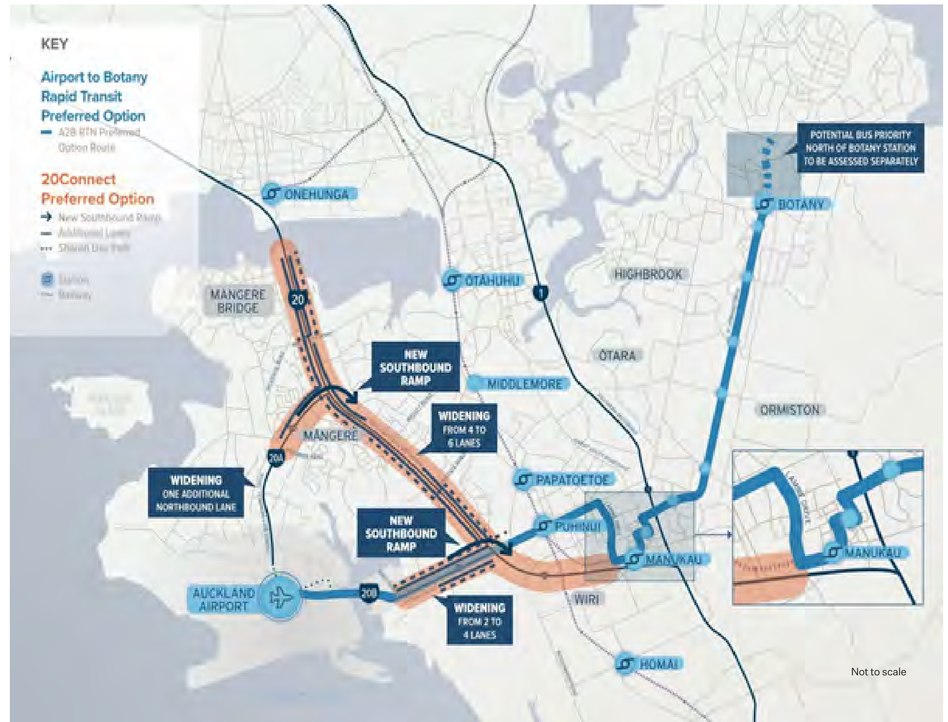
Figure 2 - Southwest Gateway project elements
