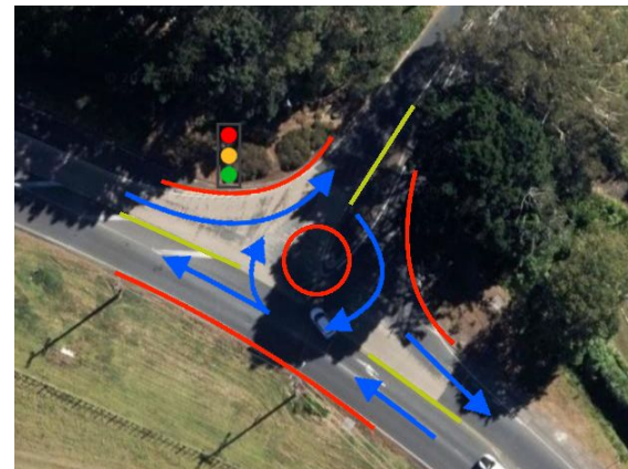
Basic Roundabout + Traffic Light
