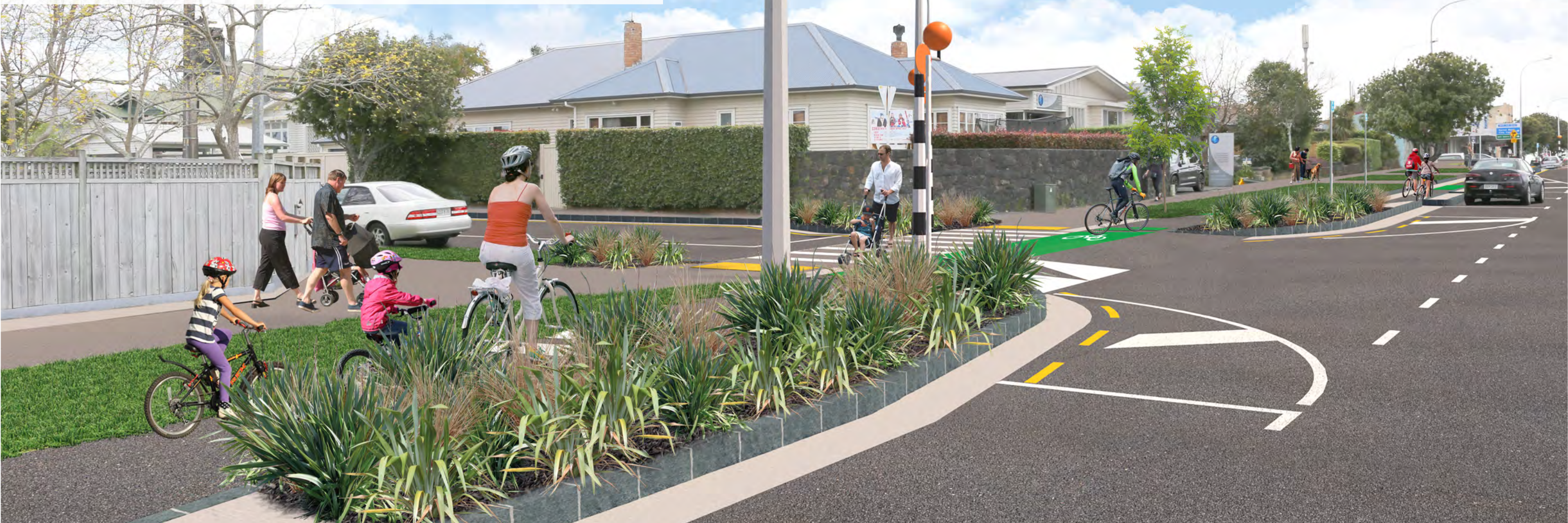
Impression of the Garnet Road separated cycleway and an improved sidestreet crossing.
