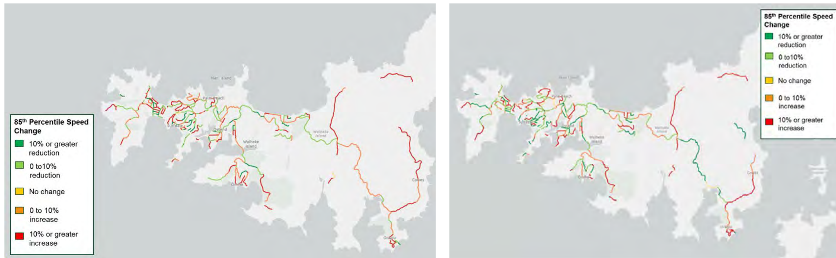
Figure E.9 Phase 1,2 and 3 85th percentile speed change (Waiheke Island- left figure is direction 1 right figure is direction 2)
