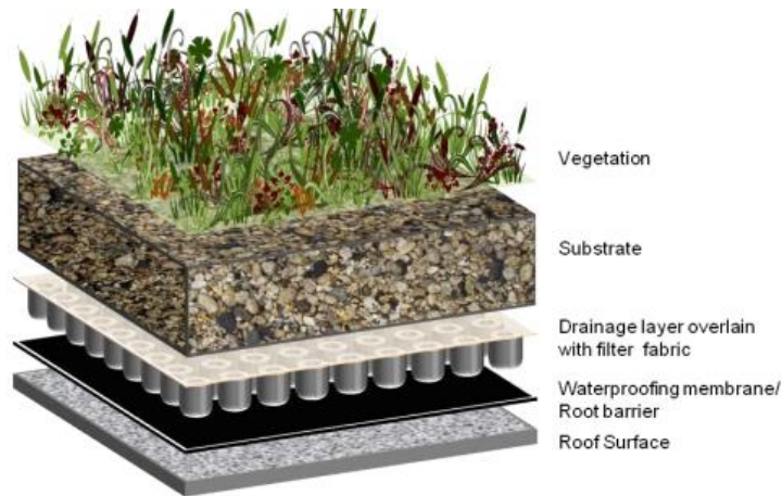
Figure 9: Typical Green Roof Composition (Auckland Council , 2013)
