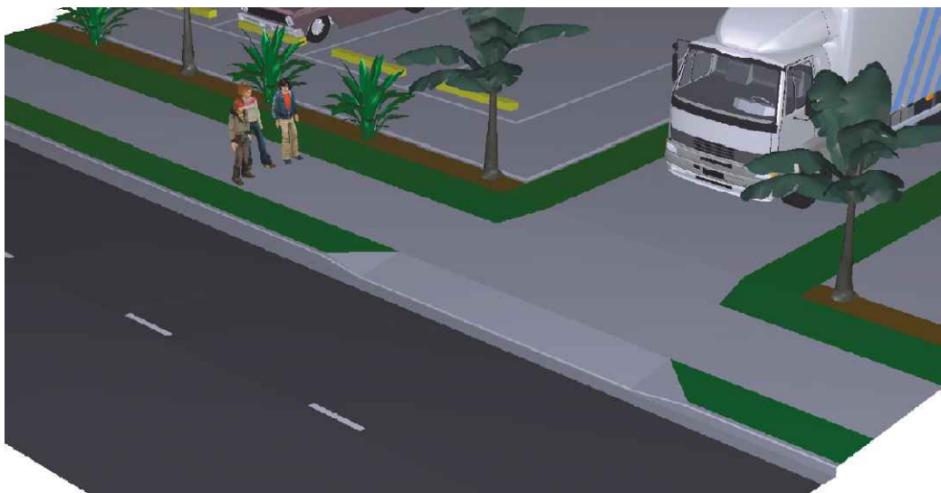
VEHICLE CROSSING FOOTPATH SEPARATED FROM KERB
