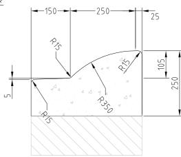
EXTRUDED MOUNTABLE CONCRETE KERB & STUB
