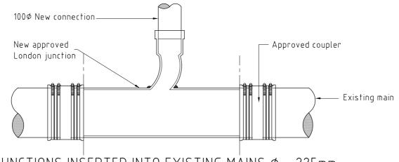
JUNCTIONS INSERTED INTO EXISTING MAINS  $\phi$  < 225mm
