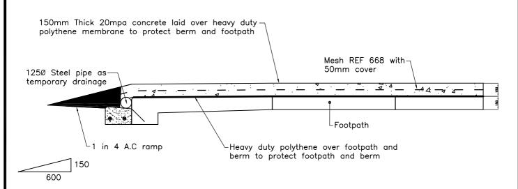
Asphaltic Concrete should be Mix 10 in accordance with Tranzit NZ Specification
