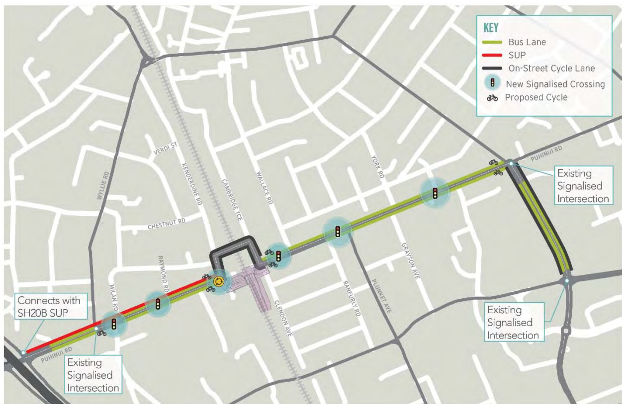
Figure 8-5: Puhinui Road Bus Priority Improvements
