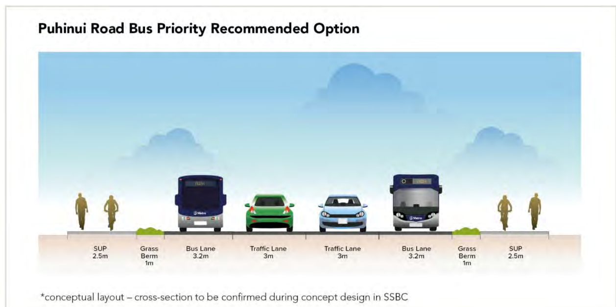
Figure 6-19: Puhinui Road Bus Priority Recommended Option cross-section
