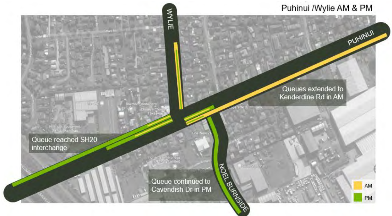
Figure 6-5: Puhinui Rd / Wyllie Rd queue analysis
