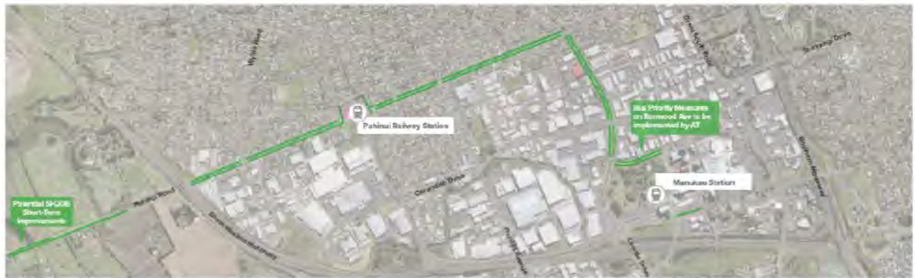
Figure 6-17: Option 3: Targeted Bus Priority Measures between SH20 and Manukau
