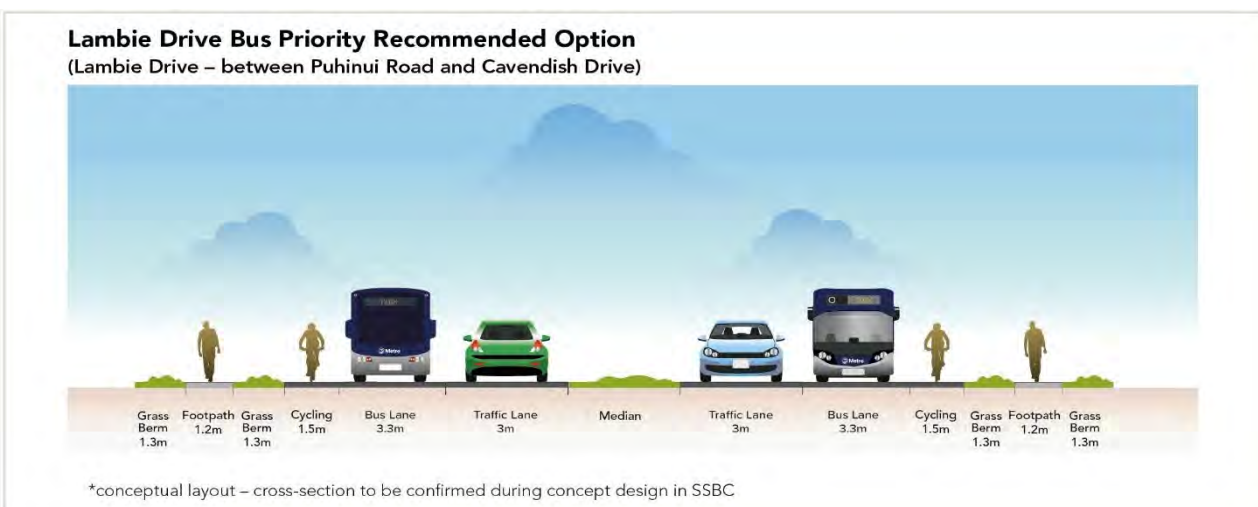
Figure 6-20: Lambie Drive Bus Priority Recommended Option cross-section (north of Cavendish Drive)
