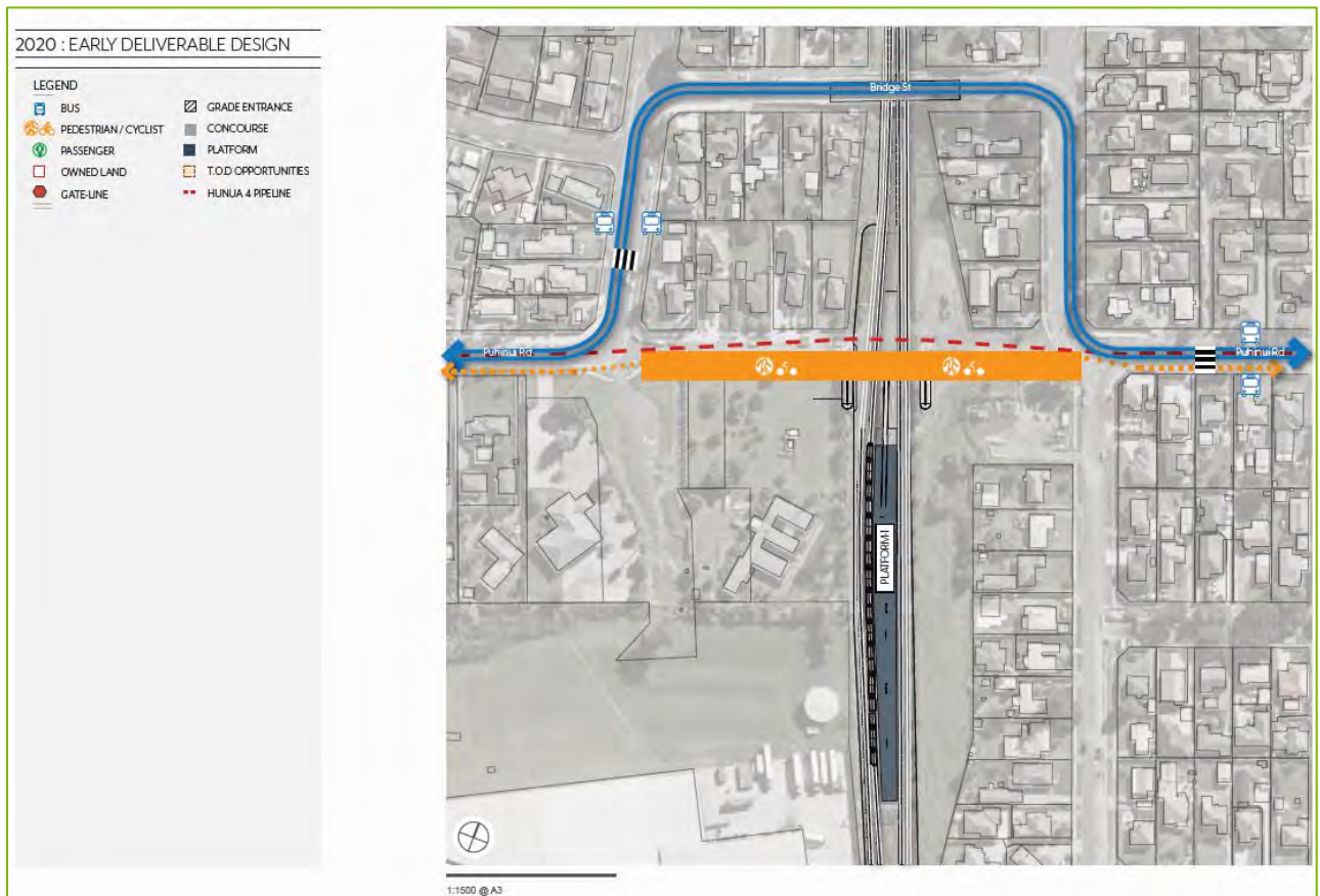
Figure 4-13: Option A: Upgraded Pedestrian Overpass
