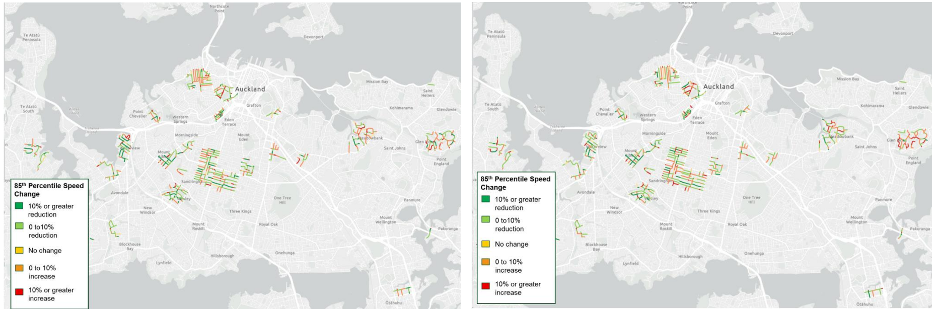
Figure E.9 Phase 2 85th percentile change (Auckland City- left figure is direction 1 right figure is direction 2)
