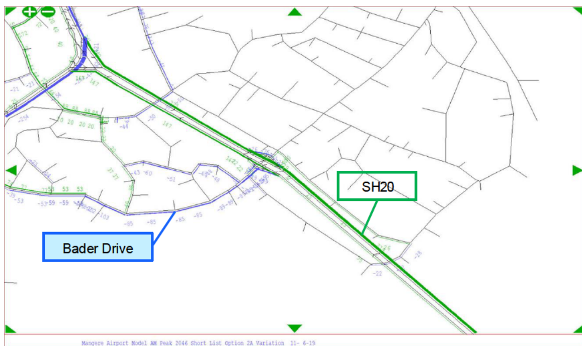
Figure 17: Bader Drive upgrades - AM traffic flow difference (combined test minus reference case)
