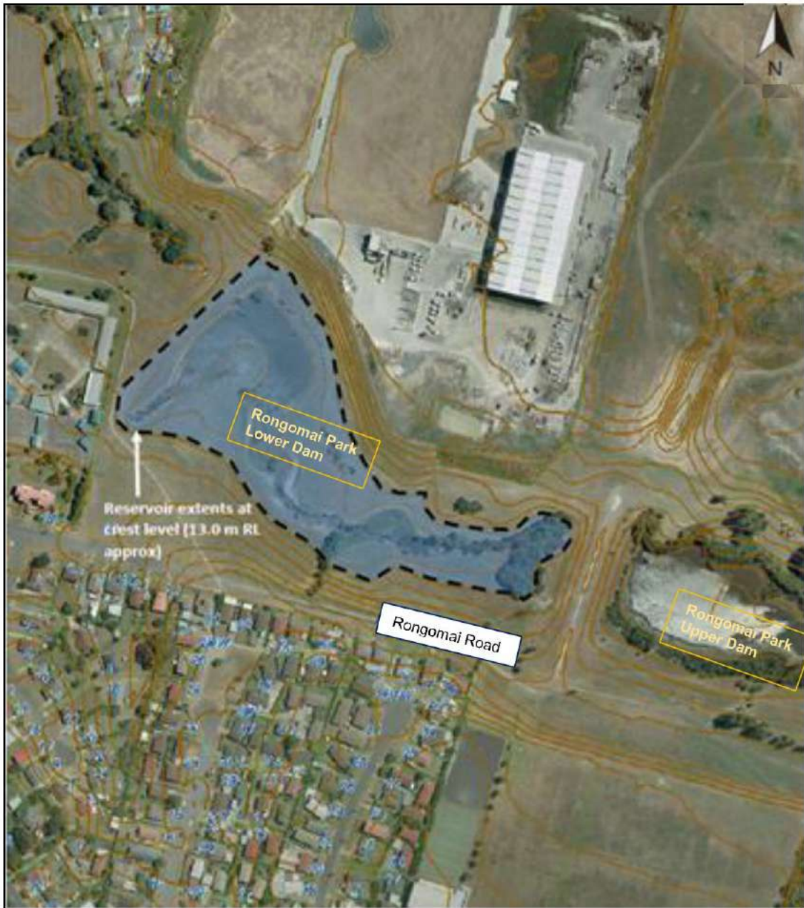
Figure 2 : Rongomai Park Lower Dam extension when water level is at the dam crest (Source: Tonkin&Taylor Rongomai Upper and Lower Dams Routing Analysis Report (2010))
