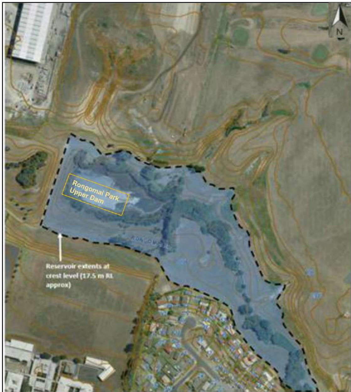
Figure 1 : Rongomai Park Upper Dam extension when water level is at the dam crest (Source: Tonkin&Taylor Rongomai Upper and Lower Dams Routing Analysis Report (2010))
