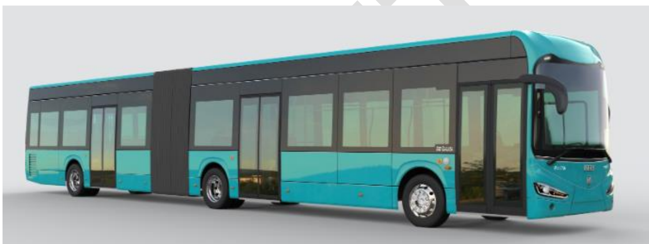
Figure 6-1: An example of an 18m articulated, low floor vehicle
