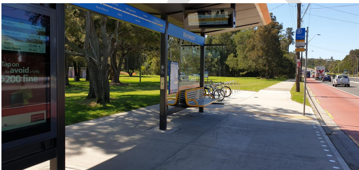
Figure 8-3: Example of station environment with shelter, seating, information, generous paving and cycle storage with kerbside bus/transit lanes (B-Line, Sydney)
