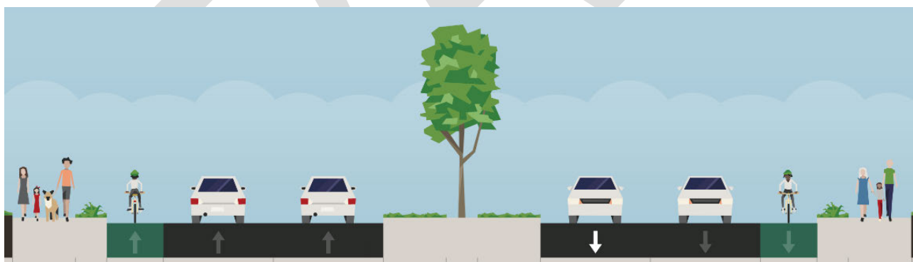
Figure 9-16: Typical existing cross section on Lambie Drive with cycle facilities
