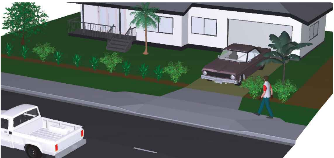
VEHICLE CROSSING WITH FOOTPATH <1.8m
